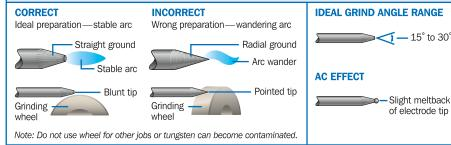
Tip: Blunting the tip of the electrode is sometimes done to help maintain consistent geometry and resist tungsten erosion. This is especially helpful in AC when melt-back of the tungsten electrode is common.
