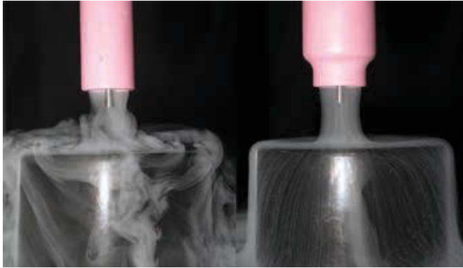
Figure 18 – Erratic Gas Flow On A Collet Body (Left) Smooth Directed Gas Flow Of A Gas Lens (Right)
