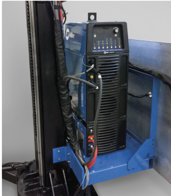
Power supply mounting rack off of the column base provides a convenient mounting space for the welding power supply, helping minimize the unit's footprint.
