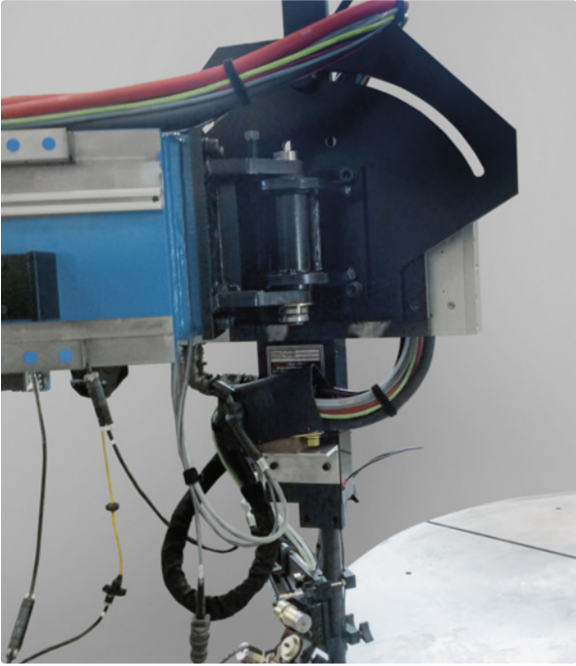
Swivel tilting brackets (left) and rotary tilting brackets (right) are available to allow precise torch positioning while welding.
