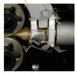
**Gun locking tab** works with guns having corresponding locking grooves to prevent gun from being pulled out if the feeder is dragged by the gun.
