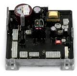
Potted and trayed main printed circuit board for the harshest environments adds exceptional reliability. Board has full-trigger isolation so a shorted gun trigger will not affect feeder operation.
