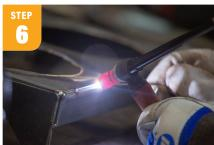
Tack weld the top, sides and ends of your stand together using a TIG welder and stainless steel rod.
