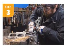
Next, clamp the ends together and use a flap disk to clean the rough edges and ensure they are symmetrical.
