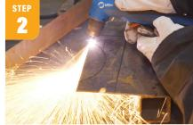
Mark cut lines for the two ends of your stand on mild steel plate and cut out with plasma cutter. The dimensions for the ends shown are 7-5/8" x 2-1/2".
