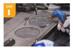
Measure the outer diameter of your bowls just below the lips they are going to rest on. Mark cut lines for circles and outer edges on stainless steel plate. Cut out with plasma cutter. Be sure to leave some extra material on the edges so you can sand down with a grinder.
