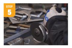
Measure and mark cut lines on the angle iron (14" in this case) and cut with a cutting wheel. These will be the sides of the stand and will give it more support.
