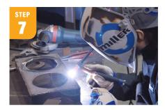
Once all of the pieces are tacked in place, use the silicon bronze rod to TIG braze the seams. You can do this using either AC or DC TIG — both were used on the stand shown.
