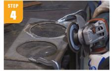
Clean the outer edges of the stainless steel to remove any sugaring. Clamp piece tight to the table, making sure that the front of the workpiece hangs slightly over the edge. This helps to keep the piece straight while cleaning — and stops you from accidentally taking off too much material.
