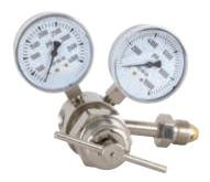
820 Series high-pressure regulators are for use on cylinders with a wide variety of non-corrosive inert gases. Piston-sensor design gives structural reliability in high-pressure use. Low-torque-control adjusting screw permits easy adjustment of pressures in closed or dead end systems.
