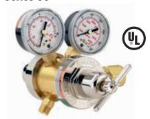
Series 30 two-stage regulators drop cylinder pressure to working pressure in two stages for consistent and accurate outlet pressure and flow regardless of inlet pressure. Recommended where outlet pressure and flow must be maintained without variation.
