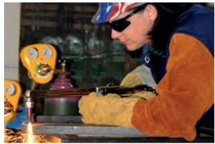
Note: Cutting capacity with tips supplied in HBAS outfit is up to 1-1/4 inches (32 mm). Cutting capacity with tips supplied in HBAS outfit is up to 5/8 inch (16 mm).
