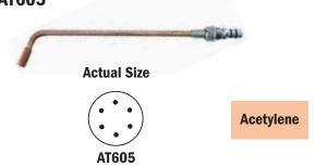
Handy light-duty multi-flame tip for heating, brazing and applying hard facing metals. Uses medium pressure acetylene and oxygen. Heads are manufactured from solid copper.
