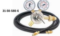
Single-stage flow gauge regulators are compact and feature a forged brass body with 2-inch diameter gauges and a self-reseating pressure relief valve. They also include a Sure Seat $^{\text{\tiny{M}}}$  protective inlet filter and a durable neoprene-composite diaphragm.
