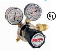
Our single-stage nitrogen regulator is specially designed to meet the specifications of HVAC refrigerant purging applications. This regulator is used with nitrogen to test HVAC systems to locate leaks and to purge an area for installation and repair. Its compact size is suitable for use where space is limited.
