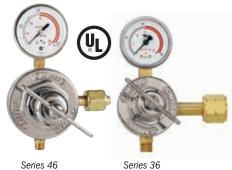
Series 46 and Series 36 brass line regulators are rugged, accurate and corrosion-resistant with shatter-resistant polycarbonate gauge lenses. The Series 46 regulators feature a stainless steel diaphragm and 2.5-inch (64 mm) gauges while the Series 36 has a neoprene composite diaphragm and 2-inch (51 mm) gauges.
