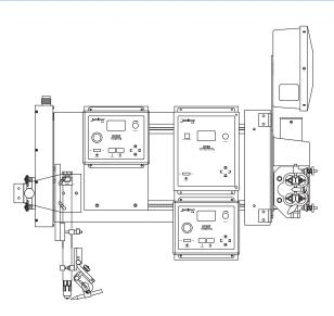
**TIG setup.** The 9700T can be installed on new or existing Jetline longitudinal seam welders and circumferential welders. The 9700T integrates with the Jetline hot/cold wire feed systems, arc length control, Weldcraft TIG torches and Miller Dynasty or Maxstar power sources to provide a complete automated TIG welding solution.
