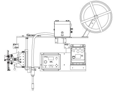
**MIG setup.** The 9700T can be used for longitudinal or circumferential welding systems for MIG. The 9700T is combined with Tregaskiss automated MIG torches, Miller MIG power sources and Jetline circumferential and longitudinal seam welding systems to provide an automated MIG solution.
