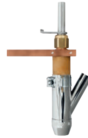
1200-Amp Twin-Wire Torch 301144 Long, 16.8 in. (427 mm) 1,200 amps at 100 percent duty cycle. For 3/64–3/32 inch (1.2–2.4 mm) wires.
