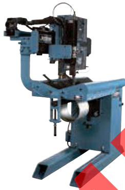
Figure 2 – A Seam Welding System
