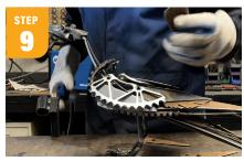
Select randomly cut pieces of sheet metal and items like saw blades, and alternate placing the pieces on each side while welding them in place, moving toward the neck and head.
