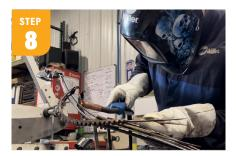
Create the bottom layer of the wing feathers with a curved scrap material and weld in place. This will be the base for the other "feathers" as you move upward.
