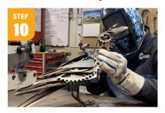
Start construction of the neck area using pieces with aggressive texture. Small sprockets or gears work well for this part.
