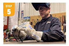
Begin by welding the legs to the table, then, once the legs are in place, construct the neck that will hold the head approximately eight inches above the legs.
