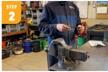
Begin by creating six-inch legs, each bent at a midpoint to form an angle between 30 to 40 degrees. Next, create assorted toe lengths, with the longest toe measuring 2  $\frac{1}{2}$  inches. Then, form the claws at the ends of the toes using small, bent nail ends.
