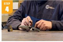
Weld the eyes to the head keeping about 3 inches distance from the tip of the beak to the eyes. Then, create the eyelids by using washers and small round stock.
