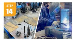
Using sheet metal, tack weld and build the drawers into a box shape that will fit the shelves.
