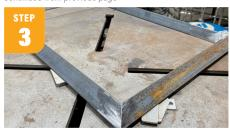
Tip the top pieces of the angle iron so they match the angle on the wood, allowing the wood to sit into the frame.
