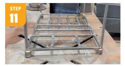
Weld the 1-1/4" diameter round stock to the four bottom corners of the table. You can drill into the bottom and add feet later to help level the table.
