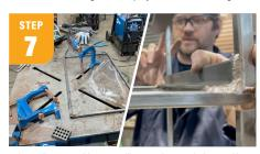
Using 1/2" square tubing, you will create the two shelves and legs of the table. For the top shelf, I cut six pieces of square tubing 6" in length. For the horizontal parts I cut them to 16-1/2" long.
