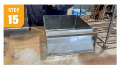
For the front of the drawer, I used stainless steel for contrast and attached 1/2" angle iron for a handle to pull it open and shut.
