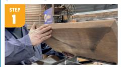
Find a piece of wood, cut it to the size you want and sand it to serve as your table top. Staining the wood is optional. You can then use this as the template for building the frame. Mine had an angled edge that allowed me to set it in a frame.
