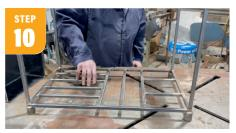
Once the top shelf and legs are created, build the bottom frame/ shelf of the table using the rest of the square tubing. I created a geometric pattern and measured the distance between each tube to keep the distance between them the same. Tack weld into place.
