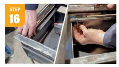
Slide the drawers into the shelves. Using the holes you made in the bar stock previously, screw in the bolts and add the anchors to set the depth of the drawer and stop it from falling out.
