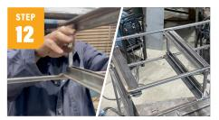
Next, create slides for the drawers to rest on and slide into. I used 1"x1" angle iron for the bottom and 3/8" bar stock for the top.
