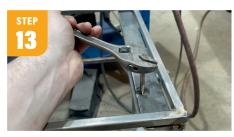
Drill and tap a 3/4" hole into the top bar stock on either side at the front of the stand to add a drawer stop later.
