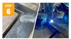
Once you have the top and bottom of the table top, weld the edges to remove any gaps in the frame and sand the edges down until the wood fits nicely.
