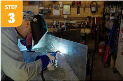
After the side panels are in place, insert the center panel to rest on the bottom of the frame. Using the Multimatic set to ¼-inch auto-set features, begin welding from the underside first, working from the center out. By spreading out the welds and dispersing heat evenly, you can help keep the fire pit square and level.
