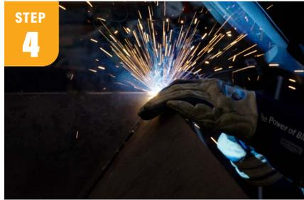
After bringing the Multimatic down to ⅛-inch settings, form and fill in the upper corners of the fire pit where each side piece meets. You will want to do this while the material is still cold. You can come back later to dress down the corners with a grinder to get a sharp edge.
