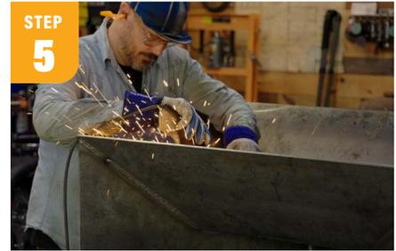
Switch the settings on your Multimatic back to ¼-inch and weld the interior corners of the fire pit from the top down to the base panel. While the area is hot, weld the base panel near the corner you just completed.
