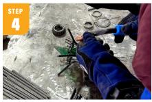
Once the rods are secured, attach more spokes parallel to the rods to fill out the sides of the torch shape. Once all spokes are tacked on, again, use the angle grinder to cut off excess materials at the bottom of the piece.
