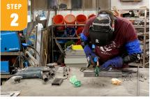
Pressure set your stone by laying a spoke over your ring and using your Millermatic 142 MIG welder to weld it to your metal ring. The end of the spoke should be pressed against the glass stone. Repeat this step two more times at equal distances around the ring so that once all three spokes are set, they hold the glass stone in place.
