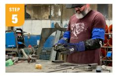
Weld another bearing to the push pins and spokes at the bottom of the piece. The spokes should fit inside the bearing, and you can hide most welds by tacking them to the inside.
