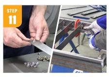
Bolt the slat tabs to the slats. Make sure the slats are level to the frame top and put two short welds on each tab inside the frame. Start the first one at  $2 \frac{1}{2}$ " and then 3" spaced for the rest.
