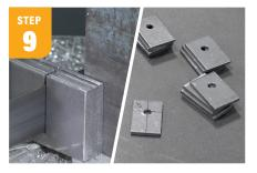
Cut sixteen, 1' x 1  $\frac{1}{2}$  piece out of  $\frac{1}{8}$ " flat stock for the cutting slat mounting tabs then drill a  $\frac{1}{4}$ " mounting hole  $\frac{1}{2}$ " x  $\frac{1}{2}$ " from one end.
