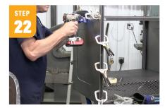
Cut 2 pieces 24 x 30" and 2 pieces 20 x 23  $\frac{1}{2}$ " for the side panels then screw the short sides on just the top and bottom with the #8 x  $\frac{1}{2}$ " self tap screws. 2 bottom sides by the basket should be  $\frac{1}{2}$ " short.
