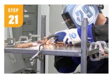
Now clamp the panel to the underside of the sq tubing and spot tack it in from the top side every couple inches.
