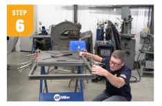
Clamp frame to the bottom of the ArcStation<sup>™</sup> 30FX and double check that it's parallel to the table. Now transfer punch the mounting holes for drilling and tapping.
