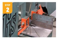
For bolting to the table, use six 3% " fine thread bolts, and cut 1% " wall 5% DOM tubing to  $1\,\%$ " for crush tubes.
