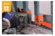
Use .063" thick 1 x 1 sq tubing for the frame. Start by cutting 2 pieces 28" and 2 pieces 20" with a 45 degree cut at each end. This will be the top.
