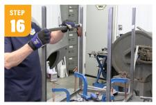
Take 2 of the 26" parts and tack in place 24" outside to outside from the top. Do the same for the two, 18" pieces, rechecking for squareness along the way and finish weld the frame.
