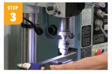
Using a carbide cutter or a bi-metal hole saw, drill three, 5/8" holes through the 1" side of the 43" long pieces at 4", 16" and 22" from the straight cut end.
