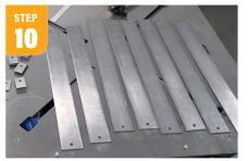
For the 8 slats, use 2" cold rolled  $V_6$ " flat stock and cut them to 18" then drill a 5/16" hole 1" from either long edge and  $V_2$ " from each end.
