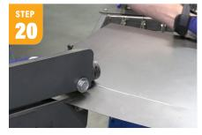
Starting with a 20" x 28" bottom panel, cut 1" x 1" off the corners so it will fit inside the legs. Option to put a step roll into all the panels to stiffen them up.
