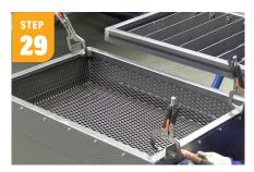
Cut the  $\frac{1}{2}$ " flat stock into 4 pieces,  $1\frac{1}{2}$ " x 2". On the top of the cabinet, weld these guide plates on the short side corners that have  $\frac{1}{2}$ " lower side panels than the long sides then use adjustment hammer or grinder to make sure they fit loosely along the cutting table top when sliding the cabinet under.
