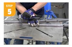
Grind the mill scale off all the weld joints, square up the sides and tack weld inside and outside corners only. Don't weld solid yet.
