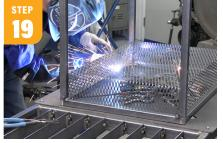
To weld the basket, leave the Multimatic<sup>®</sup> Auto-Set<sup>™</sup> setting to 16 ga, pull the sides out a little and weld them to the top of the 1x1 sq tubing.
