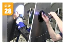
Clean-out ports come in many sizes. For the RV/ boat style, cut about a  $5 \frac{3}{4}$ " diameter hole (2  $\frac{7}{8}$ " radius) to fit clean-out port, then drill holes and secure with sheet metal screws.
