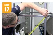
Check for squareness by taking some diagonal measurements. They should read the same. Because you didn't weld any of the outside seams, the panels will fit flat.
