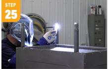
Weld the leveler bolts in. Use %"-16 fine thread x 1 %" long bolts with a thin jam nut and a standard nut that is TIG or MIG welded in the end of the 1 x 1 legs. Remember to grind the plating off your nuts.
