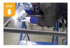
Bolt the frame to table, double check that it's level and weld the outside and inside joints. Do not weld the top or bottom seams.
