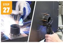
The exhaust port is a 4" long piece of tubing that the FILTAIR<sup>®</sup> hose will fit tightly inside. Cut a hole in a 4  $\frac{1}{2}$ " square piece and spot-stitch halfway onto the tubing. Then cut the same hole in the side of the cabinet, centered about 7  $\frac{1}{2}$ " up from the top edge and secure with rivets or screws.
