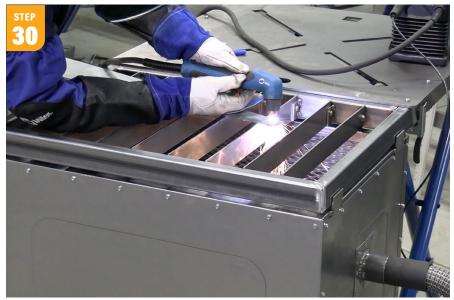
Lastly, hook up exhaust port hose, turn FILTAIR® 130 up to maximum vacuum and start cutting.
