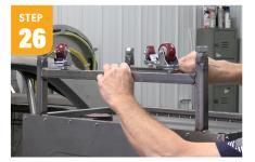
The size of the wheels will determine the position of the cross bar. If you use 2" diameter wheels with a 3%" x 1" mounting stud, the cross bar will be 32 ½" from the cabinet top but wheels are still adjustable. The bottom of the cutting table is about 33" from the floor and you need clearance to slide under it. Use weld nuts or riv-nuts to mount wheels.
