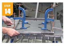
You will basically be building this upside down. Square the top, clamp and weld the inside and outside corners while still avoiding welding the top or bottom. Grind the outside corner welds flush so the panels will fit tight and Auto-Set <sup>™</sup> welder to 16ga.
