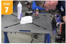
Remove clamped frame to drill holes. Move the rear leg mounting bracket to drill the back holes. Use a letter Q drill bit and  $\frac{3}{6}$  x 24 fine tap.
