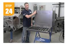
Then weld the two 6 ½" pieces 2 ¼" in on each side of the bottom frame. This will clear the Folding ArcStation™ 30FX front legs.
