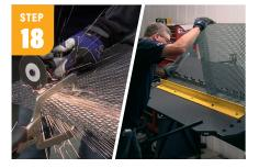
Make a small parts catch screen using expanded metal that's about .070" thick. Overall measurement is 34" x 26" and trim 4" x 4" off each corner. Bend into a box frame.
