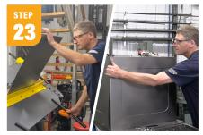
For the 30" panels, bend about a 1" lip on each short side to overlap the panel next to it. It's optional but saves a bunch of screws and it looks cleaner.
