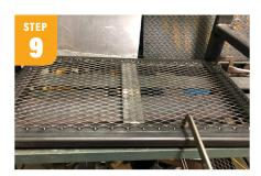
Set the expanded steel grating (  $37" \times 19" \times .13"$  thick) on the top of the base (seat). Square up all sides. Clamp down your base in a few spots to keep it in place, then tack all points down on all four sides. This secures the expanded steel to the base and also removes/covers any sharp corners and edges. Paint the swing or leave as is.
