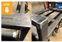
Take the 3" x 6" x .13" hot rolled flat and cut into (2) 3" x 3" pieces. Grind down the welds on the armrests, then place one 3" x 3" piece on each armrest to cover the ends. You can choose to grind the welds for a smooth appearance or leave it to achieve an "as welded" look.
