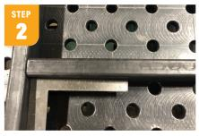
Each armrest has (2) 20" tubes and (1) 8.5" tube. For each armrest: Lay one 20" tube vertically (this is the back of the armrest). Measure up 7" from the bottom and make a mark. Lay your second 20" tube horizontally, making a sideways "T". The bottom of the horizontal 20" tube should rest where you made your mark on the vertical 20" tube.
