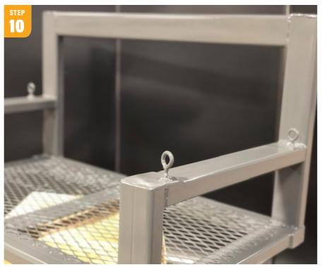
Get your desired length of chain and clevis pins to mount your swing. Note: The size of the pin must be small enough to slide through the eye bolt. Find a sturdy place to screw in your eye bolts (such as a rafter, beam or frame), and mount your swing. Sit back (literally) and enjoy.
