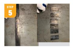
Take the 1.5" x 18" x .13" hot rolled flat and cut into (6) 2.75" endcaps. Cover each tube's opening (except for the two armrest tubes) with an endcap and weld it down on all sides.
