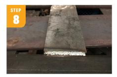
Take the steel plate (3" x 17" x .19" thick) and place it vertically in the middle of the base (seat). Make sure it is centered and weld it into place at the top and bottom, creating a support beam for the seat.
