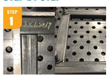
For the base (seat): Lay out 4 base tubes, (2) 40" and (2) 17", to make a rectangle. Square up the corners, and clamp down with a c-clamp or wide vise grip. Tack all joints. Flip the base over and tack all joints on the back. Note: tack joints only. Hold final welding until after step 4.
