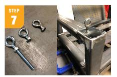
Take the (4) 5/16" eye bolts with nuts — screw the nuts all the way to the top until they reach the eye bolts. Cut just below the nut with your cutting wheel, removing the lower threads. Loosen the nuts (about one turn) and tack the inside of the nut. Tack the eye bolt until you can't see the seam. Place on the top of your armrests and weld the nut to the tube, then weld the bolt to the nut.
