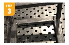
To make the front of your armrests, take your 8'5" tube and lay it vertically at the other end of the horizontal 20" tube. Make sure the horizontal tube is square with both vertical pieces of the armrest. Once set, clamp and tack joints. Repeat steps for the other armrest. Place tacked armrests on the base (seat). Make sure they are square with the front and rear of the base. Tack in place.
