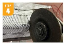
Using a cut-off wheel, reciprocating saw or plasma cutter, cut out the pieces. Leave a small amount of excess on the cut lines to allow for fine tuning later. Hint: Try to make your cuts in an order that keeps the tube as intact as possible for ease of fixturing!
