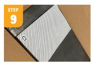
The pattern for the shelf will need to be cut from a piece of flat steel. I chose 1/8" steel.
