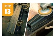
The next thing to focus on is the chimney. This could be welded up any time in this process. I tacked the pieces together at the ends and middle and then alternated stitch welds to help manage the heat. Cook's choice whether to grind these welds off or not.
