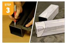
Mark the centerline of the tubes to help provide the best possible alignment of the patterns. Cut out and apply the patterns to the tubes using Super 77 spray glue (or equivalent). Apply spray glue to the rear of the pattern and to the steel to ensure maximum adhesion.
