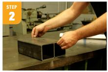
Cut two pieces of 4" x 3/16" square steel tube into 12" lengths. Deburr the edges for safe handling. Wipe down the tube inside and out with denatured alcohol to remove oils and surface contaminants. This is a necessary step for the patterns to stick to the steel. If the tube is rusty, you may want to also use a Scotch-Brite pad.
