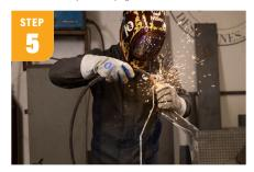
Take two of your table legs and tack weld at the top. Next, add the third leg and tack weld it to the other two. Place tack welds on the bottom where the three pieces meet. Then, adjust the legs to ensure they are correctly placed and weld together.
