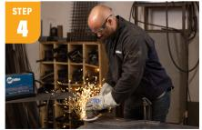
Once your legs are cut out, first use a grinding disk to clean the edges and remove any excess material, then use a sanding disk to soften the edges. If you want to give your table legs a hand-forged look, take a sanding disk and run it over the front and back of each leg.
