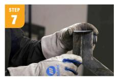
Optional: Tack weld a small disk onto the top of the table base for additional stability when mounting the table top
