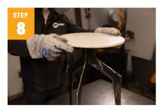
Apply a high-grade adhesive to the disk (or directly to the top of the base if you skipped Step 7) and mount the marble top to your table base.
