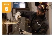
Grind down the tack welds on the top of the table base and smooth the bottom of each table leg with a sanding disk to ensure your table is level.
