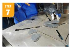
Flip four welded hearts over and weld four more hearts to the front. Welding each heart at a ~45-degree angle will give appearance of depth/3-D layering.
