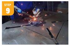
Cut, bend and weld solid rod/stem to backside of the flower.
