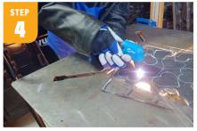
Use plasma cutter to cut hearts from the material. Clean cut hearts as desired (optional).
