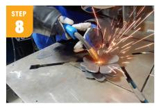
Add texture to the flower by welding a circle in the center, then weld a series of quick "tack" welds to cover.
