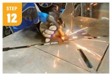
Sign the base by dropping welding machine amperage down to ~20 gauge preset settings to "draw" signature on base of flower.
