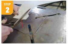
Cut out template using scissors.
