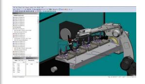
Special functions speed up programming of similar parts and welds
