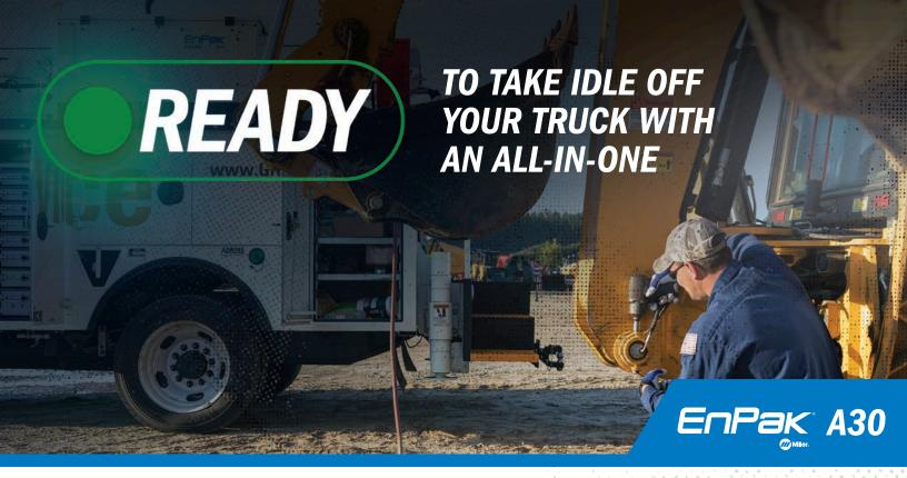
With industry-leading technologies, the EnPak® A30 takes idle off your Class 3 to 5 trucks, reducing operating expenses and giving operators the power they need to get jobs done. It delivers 210 amps of integrated multiprocess welding output, 30 cfm of compressed air, battery charge/crank assist and 6,500 watts of generator power.
