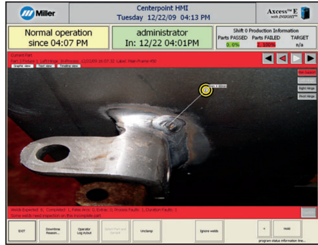
HMI View for Operator
