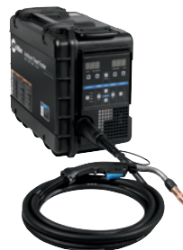
SuitCase® 12RC Wire Feeder 951580001 Lightweight and flexible enough to run wires up to .062-inch diameter. Includes remote voltage control, drive roll kit and Bernard® BTB Gun 300 A. See literature M/6.5.
